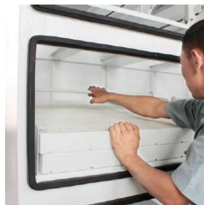
3.Put the pushrod down, fixed the filter.
