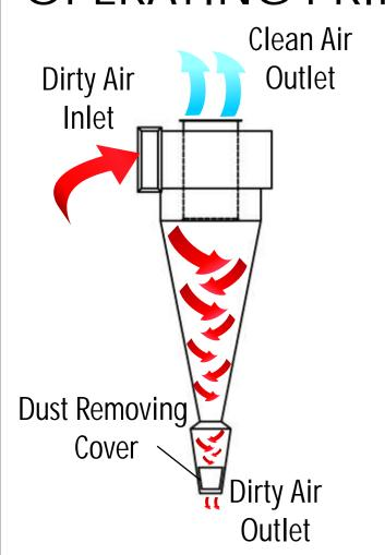
At the cyclone inlet, a helical flowing form is given by means of a cyclone construction to the dusty gas entering the cyclone tangentially with high speed and it is ensured that particles whose density is higher than the holder environment are directed to cyclone walls by the centrifugal force.
